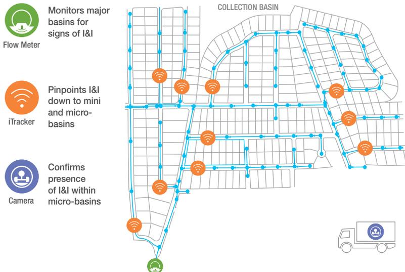
In most instances, **after just a single storm event**, the problem is pinpointed down to mini and micro basins without the requirement for expensive monitoring equipment, confined-space entry, repetitive maintenance or "in the road" data retrieval. This single storm approach is the main factor when it comes to delivering a successful and cost effective I&I detection study.
