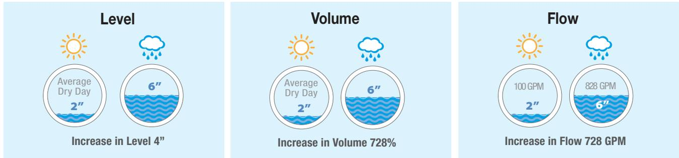
This is where iTracking® delivers huge benefits. By having the ability to simply convert level readings recorded by iTracker® sensors to actual changes in volume and then ultimately to flow in gallons per minute, a safe, quick and cost-effective solution is now available to every community, regardless of size, for pinpointing I&I down to a pair of adjacent manholes.
