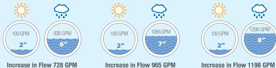
iTracking® analytical software converts percentage changes in wastewater volume to flow in gallons per minute.
