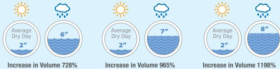
Smart algorithms calculate percentage changes in wastewater volume between the average dry day norm and wet weather events.
